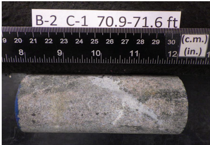
After cutting and grinding
