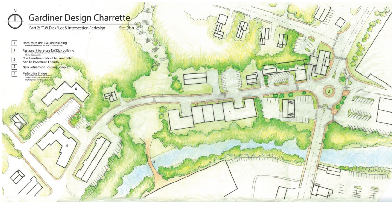
Proposed reuse of the TW Dick property with a rotary to provide safer pedestrian crossing on Bridge Street
